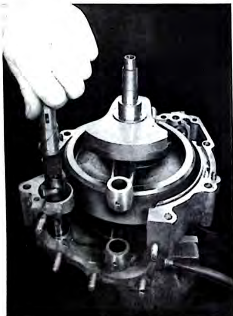
FIG. 23 Fitting the Camshaft
