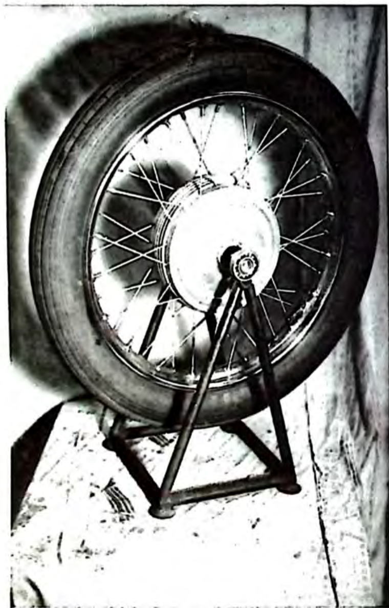
FIG. 46A Balancing the road wheels
