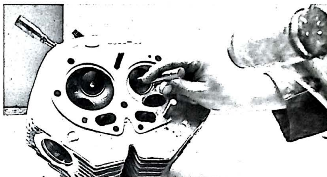
Fig. 12. Drifting Out Valve Guide.
