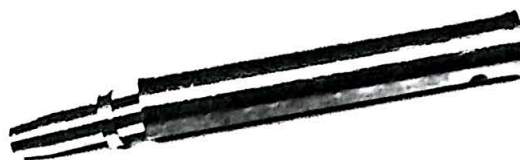
Fig. 11. Valve Guide Fitting Tool.
