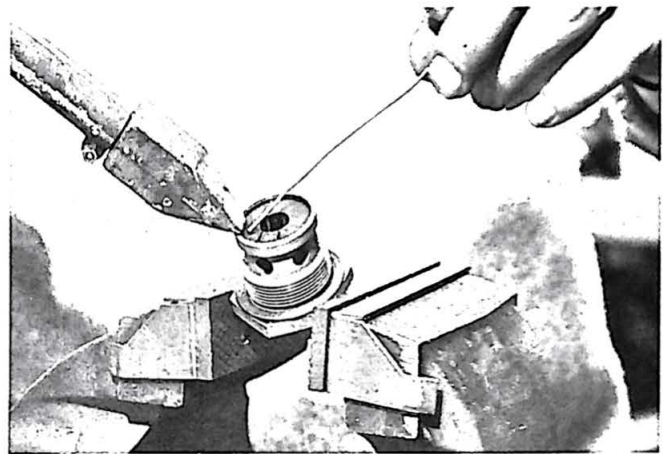
Fig. 44. Soldering Circlip into Sump Filter.
