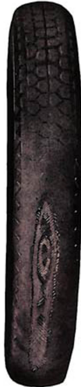
Illustration shows excessive wear through high spots in brake drum
